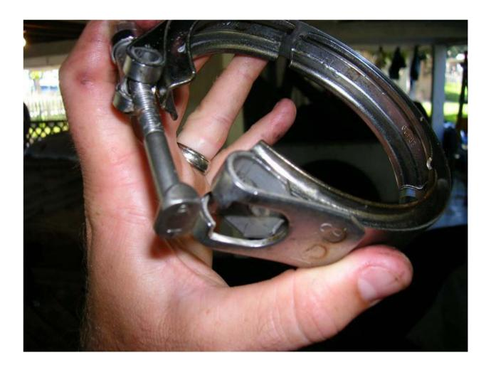
Once you have the clamp off, it'll make it easier to move the exhaust back if you also unhook the small (about  $\frac{3}{4}$ ") hose from the top of the J-pipe to the exhaust manifold.
