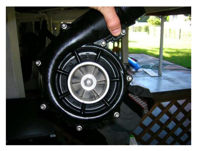
If you have an adapter installed on your supercharger to connect to an aftermarket air intake, remove it at this time and set it aside.
