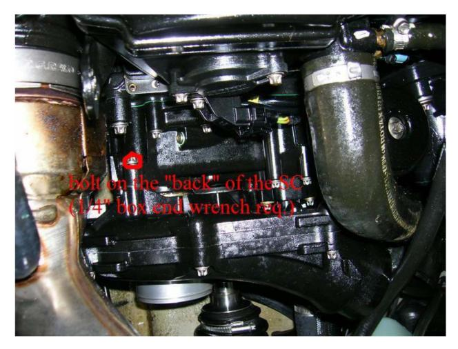
Once you have the three bolts off you can carefully slide the SC out. Once again, be careful. You do not want to damage any of the surfaces of the shaft, housing, or gear. Doing so will be big \$ and bigger headache.
