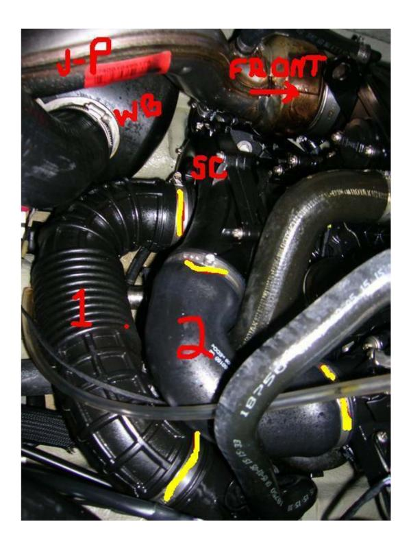
Then remove the hose between the SC and the throttle body (#2). If you have factory (Oetiker) clamps as I do then you'll have to buy replacements as these get ruined and are not reusable. (Hose clamp is included in your kit so don't worry about damaging the 1 Oetiker clamp) Only remove the Oekiter clamp that is attached to the supercharger and not the intake. Even though it's a bit of overkill unless you're
