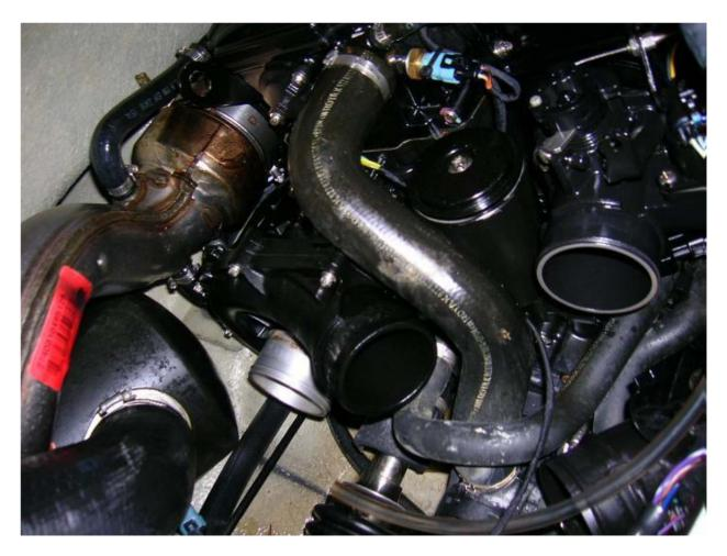
Now it's time to move the J-pipe and waterbox back just a couple inches to give you room to work and provide the required space to pull the SC out once you've unbolted it too.
