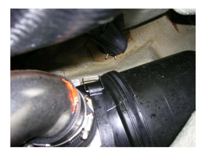
Once you unhook the J-pipe, hose, and waterbox you can slide the entire exhaust assembly back about 2-3 inches. Be careful, as there is still a hose attached to the bottom of the J-pipe, so don't force it. I prefer to unscrew one of the hose clamps allowing me to completely slide the j-pipe back allowing more room for you to remove the supercharger. This is also a good time to check the bilge for anything that can block the bailer tubes. Check for leaves or nuts and bolts.
